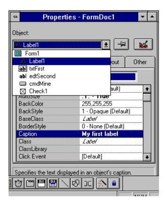
Figure 1 Object Dropdown - You can move from a property of one object to the same property of another just by choosing the new object in the dropdown.
